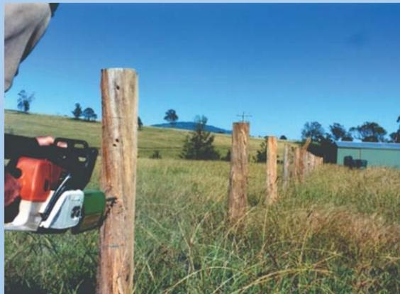
**ABOVE:** An Atom drilling attachment fitted to a conventional chainsaw makes easy work of a hardwood post.
