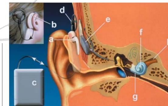
ABOVE: The Cochlear implant: (a) microphone; (b) behind the ear speech processor; (c) body worn speech processor; (d) transmitting aerial; (e) receiver stimulator; (f) electrode bundle; (g) inner ear (cochlear); (h) auditory nerve. TOP: manufactured components ready for installation.
