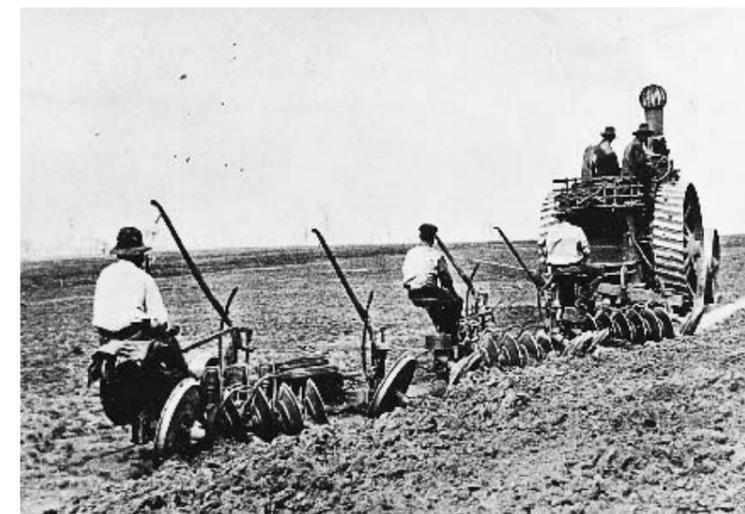
ABOVE: Stump jump disc ploughs near Tamworth in 1915. Generally disc ploughs are efficient and economical. In this photo they are part of a remarkably labour intensive process for cutting a furrow.
