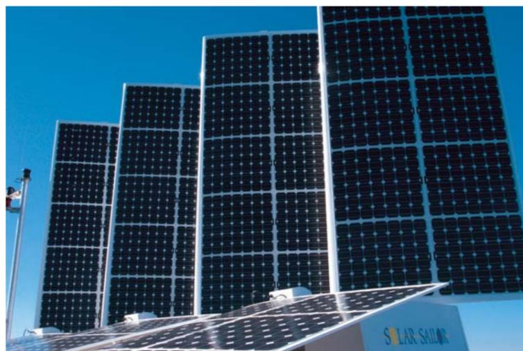
ABOVE AND OPPOSITE: *The Solar Sailor*, built in 2000 by Advanced Technology Watercraft, is a cruise vessel for 100 passengers. It runs on a combination of solar power, wind power and LP gas.
