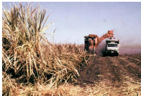
Made possible by Australian invention, automated harvesting of sugar cane has taken over from back breaking manual labour in recent decades.
