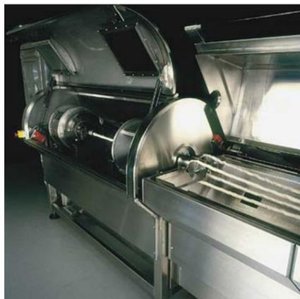
*The Optim wool fibre processing machine, designed by Invetech Operations. Introduced in 2001, it is the manufacturing apparatus for the latest enhancements to wool fibres developed by the CSIRO and the Woolmark Company. It produces luxurious lightweight fibres suited to all seasons, and is one of many Australian developments that boost the value of our wool clip by keeping wool and wool blends a few steps ahead of synthetic fibres.*
